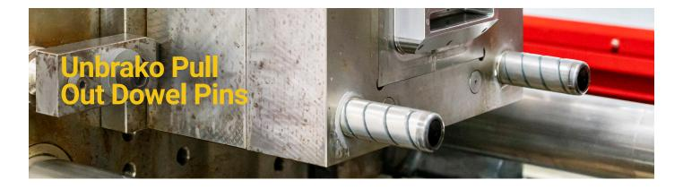
Unbrako's line of Pull Out Dowel Pins are designed with a unique spiral groove that releases trapped air when being inserted into its application. This spiral groove ensures an easier installation, and the tapped hole in one end makes removal faster and eliminates the need for additional knockout holes.
