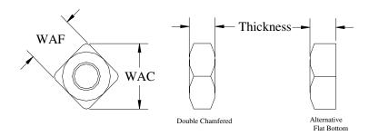
The physical and material properties of the nuts are made to the requirements of the Society of Automotive Engineers standard SAE J995 as specified for grade 5 hex nuts:
