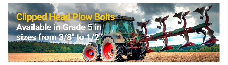
Most often used on heavy tractors & agricultural equipment — Clipped Head Plow Bolts are designed to attach plow shears to agricultural plows, allowing the tractor to churn up dirt and break up the soil. These bolts feature a flat round head with trimmed sides which prevents the bolt from loosening once tightened. Earnest Machine stocks Clipped Head Plow Bolts in Grade 5 with diameters ranging from 3/8" to 1/2" and lengths ranging from 1 1/4" to 1 1/2".
